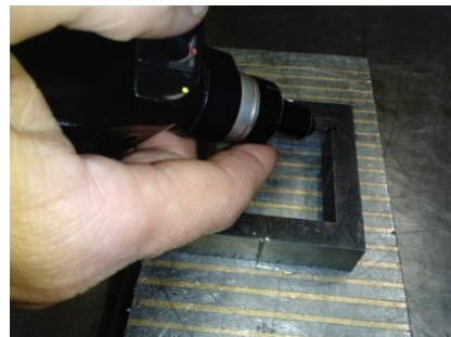
Figure 9. Measuring the exterior surface cut by abrasive water jet (AWJ)
