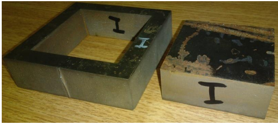
Figure 6. 1C45 steel part cut with abrasive water jet (AWJ)
