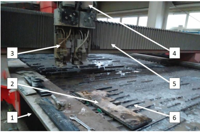
Figure 2. Elements of the abrasive water jet machine
