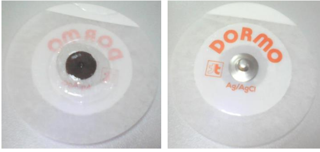
Figure 4. Ag/AgCl electrode used for recording (left - front, right - back)
