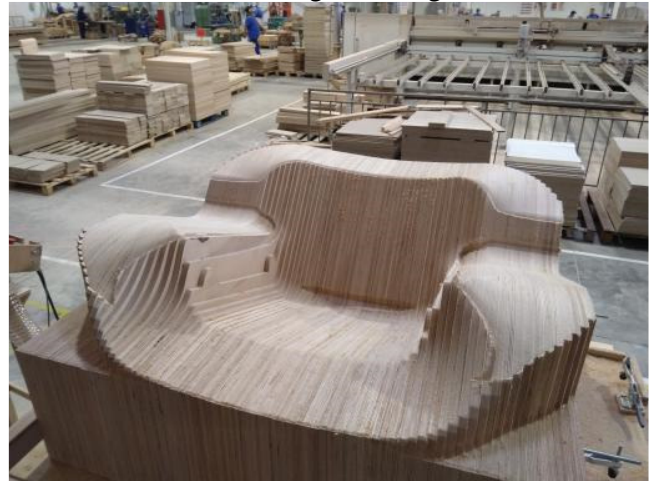
Figure 13. Cavity finish milling
