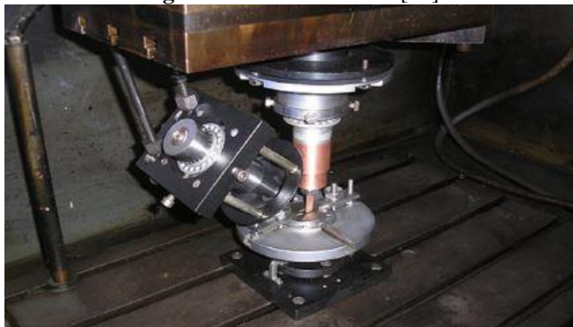
Figure 9. Ultrasonic chains for EDM+US microslots [19]
