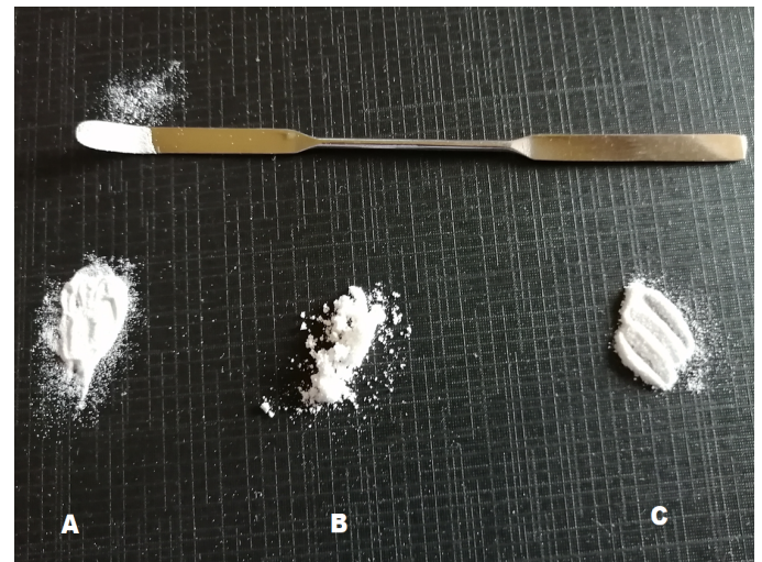
Figure 8. PA2200 Powder A – Reference material; B – Contaminated material; C – Decontaminated material
