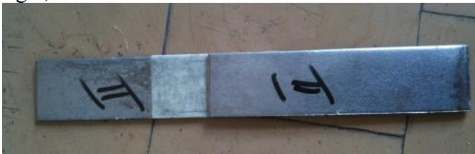
Figure 6. Assembly made in order to carry out the shear test [14] (normal view).
