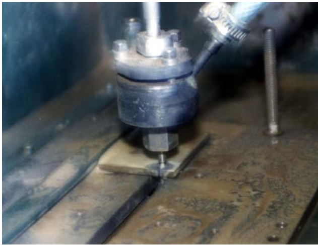
Figure 8. Abrasive water jet cutting head (ICTCM)
