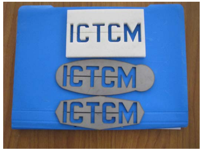
Figure 12-b. Stainless steel (6 mm) and marble (20 mm) cut with AWJ
