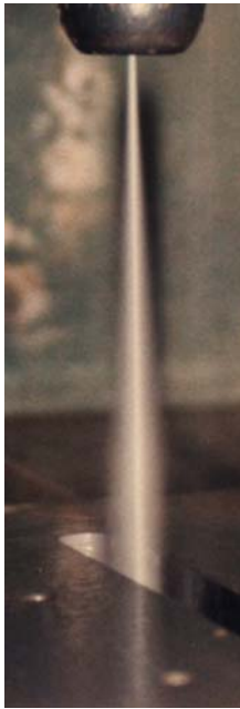
Figure 2. View of a high pressure water jet (230 MPa)
