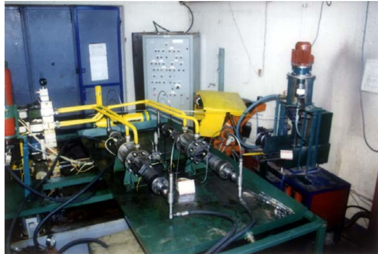
Figure 10. Abrasive water jet cutting equipment (ICTCM)
