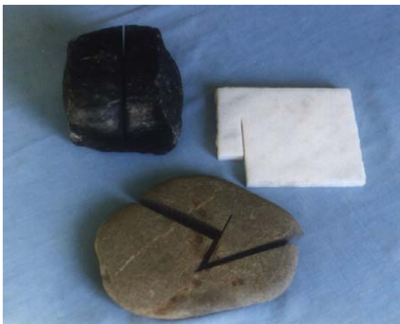
Figure 12-a. – Stone, granite and marble cut with AWJ
