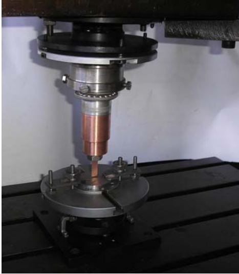
Figure 12. Photo of the equipment mounted on ELER 01 without additional ultrasonic flushing device
