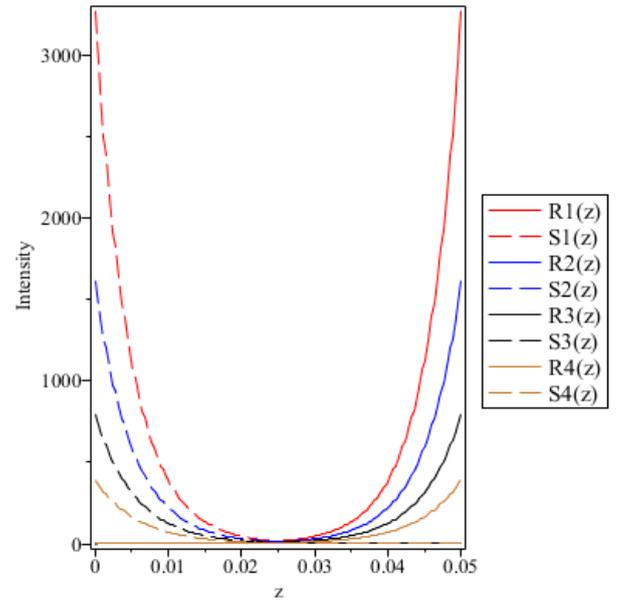
**Figure 3.** The complex wave amplitude  $R(z)$  and  $S(z)$  for four values of coupling coefficient  $\kappa$ .  $R1(z)$  and  $S1(z)$  correspond to  $\kappa = 150$ ,  $R2(z)$  and  $S2(z)$  to  $\kappa = 140$ ,  $R3(z)$  and  $S3(z)$  to  $\kappa = 130$  and  $R4(z)$  and  $S4(z)$  to  $\kappa = 120$ .
