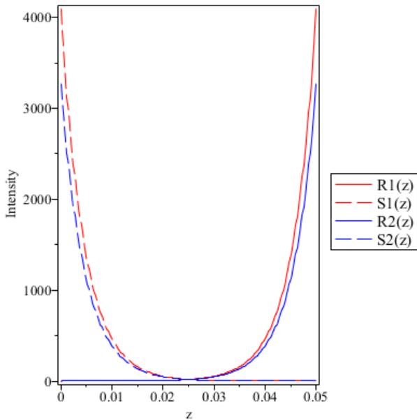
**Figure 2.** The complex wave amplitude  $R(z)$  and  $S(z)$  for two values of gain coefficient  $\alpha$ .  $R1(z)$  and  $S1(z)$  correspond to  $\alpha = 5$ , and  $R2(z)$  and  $S2(z)$  correspond to  $\alpha = 0.5$ .
