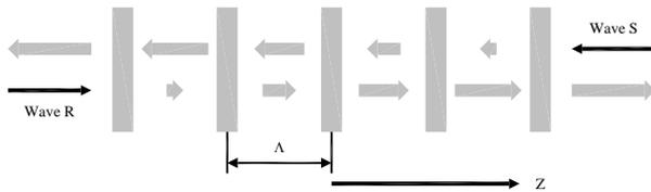
**Figure 1.** Schematic representation of the oscillation mechanism of a DFB structure. Wave R - left-to-right propagating wave, Wave S - right-to-left propagating wave,  $\Lambda$  - Bragg grating wavelength,  $Z$  - propagation coordinate [13].
