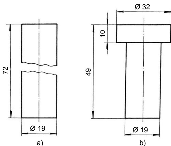
**Fig. 3. Blank's and Piece's Dimensions**
