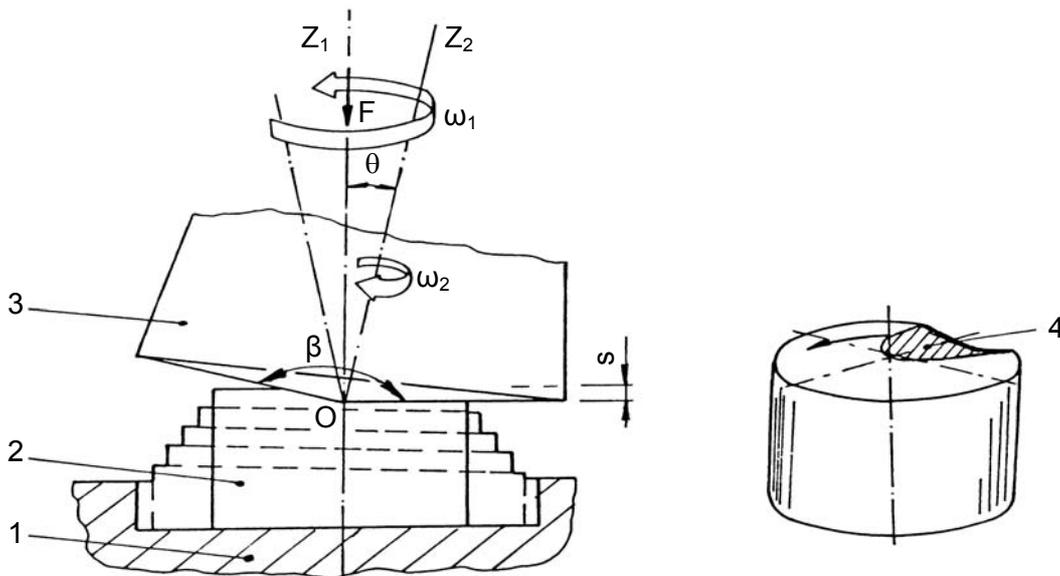
Fig. 1. Orbital Forming Process Kinematics, [1]
