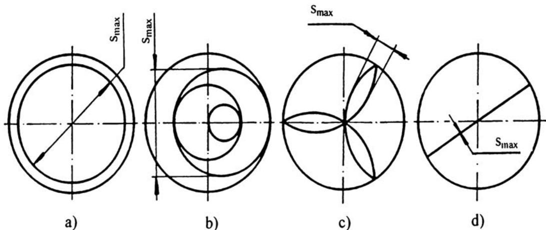
**Fig. 2. Characteristic Curves of Contact Surface between Oscillatory Die and Worked Piece Trajectory**
