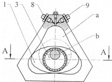
**Fig. 8. The section after plan B-B through pump.**
