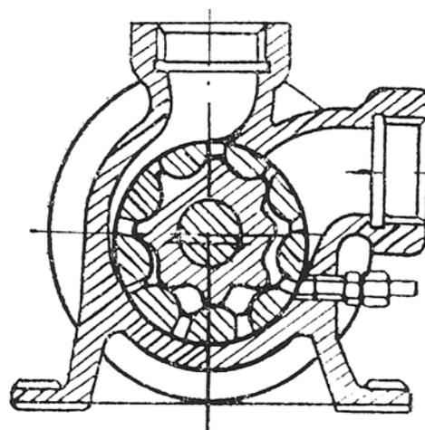
**Fig. 1. Hidraulic pump with stellated wheel.**
