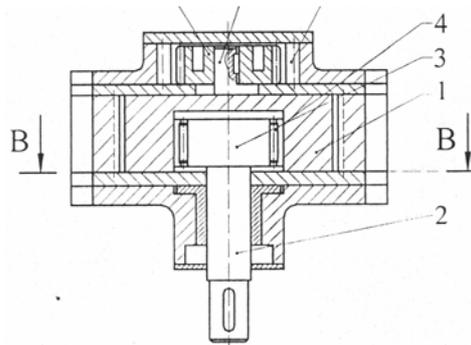
**Fig. 7. The section A-A in vertical plan through pump.**
