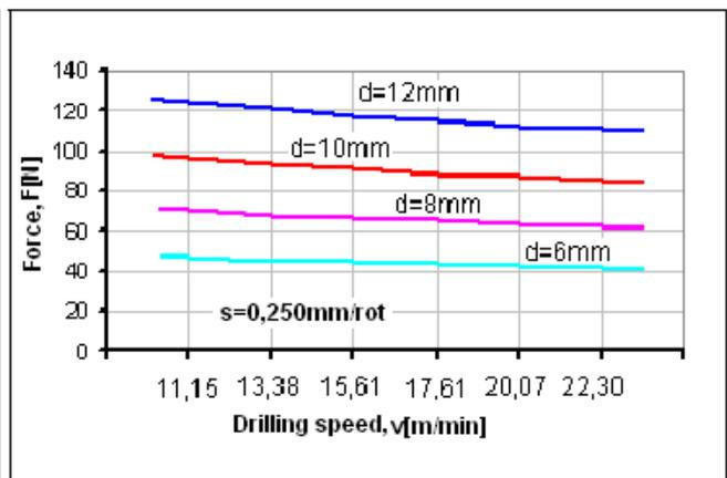
**Figure 7.** Shows the variation of axial force as a function of drilling speed, for different drill diameter ( $s=ct$ )
