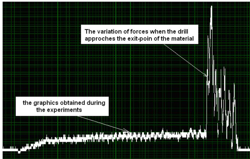
**Figure 8.** The variation of splintering forces when drilling
