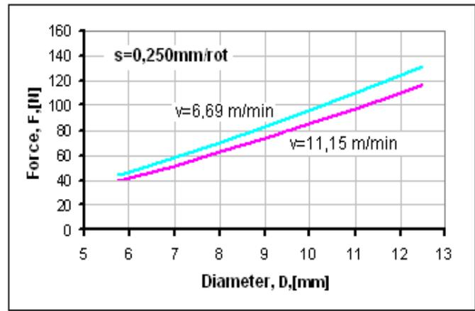
**Figure 5.** Shows the variation of axial force as a function of drill diameter, for different drilling speeds of the tool ( $s=ct$ )
