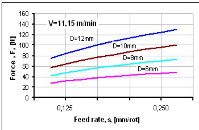
**Figure 2.** Shows the variation of axial force as a function of feed rates, for different drill diameter ( $v=ct$ )
