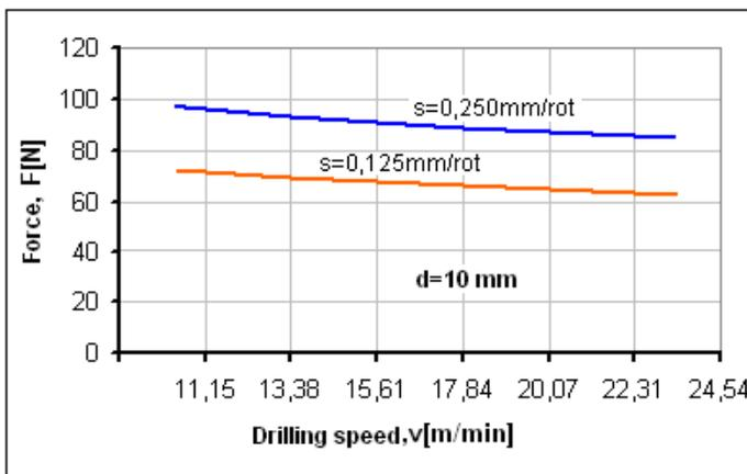
**Figure 6.** Shows the variation of axial force as a function of drilling speed, for different feed rates ( $d=ct$ )
