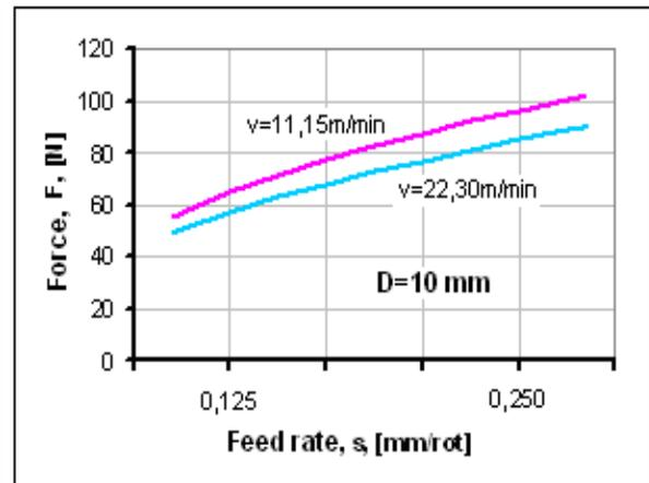
**Figure 3.** Shows the variation of axial force as a function of feed rates, for different drilling speeds of the tool ( $D=ct$ )
