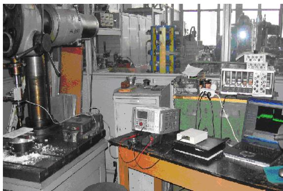
**Figure 1.** The image of the stand of determinations with the force moment pickup and the registration system
