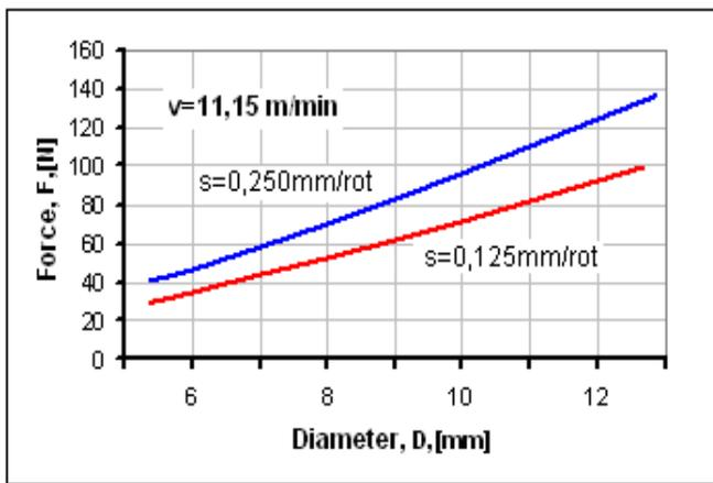
**Figure 4.** Shows the variation of axial force as a function of drill diameter, for different feed rates ( $v=ct$ )
