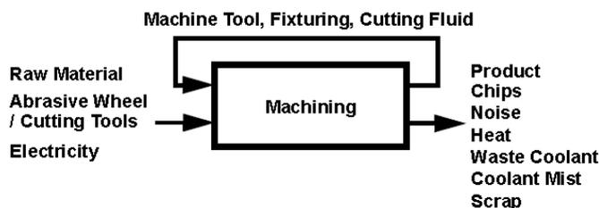
**Figure 1.** Input-Output Diagram of a Traditional Machining Process
