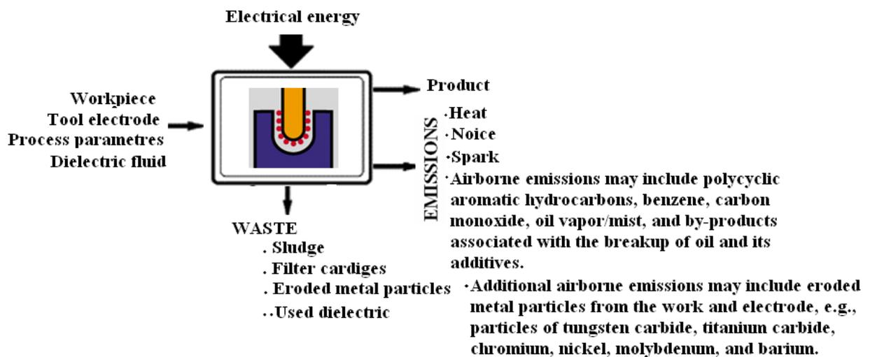
Figure 2. Input-Output Diagram of a EDM Process
