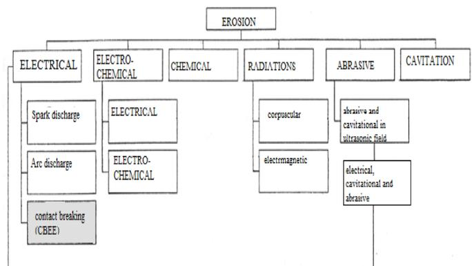
Figure 1. Main types of erosion of technological interest
