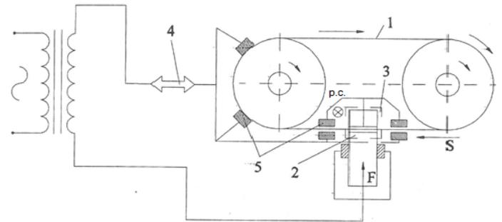
**Figure 3.** The basic scheme of CBEE principle, with T.O. – steel strip
