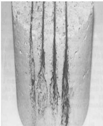
**Figure 6.** Width variation of the trace left by an abrasive grain
