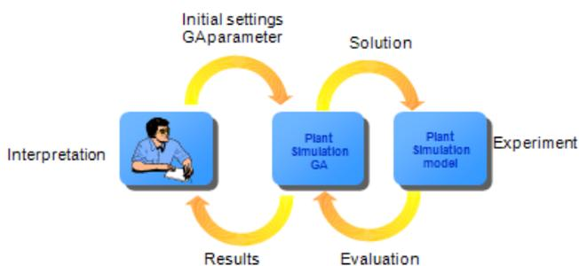
Figure 8. Iterative Optimization with Plant Simulation [10]
