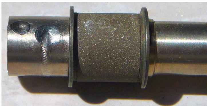
**Fig.2. Electron beam welding, made at ISIM Timișoara (detail).**
