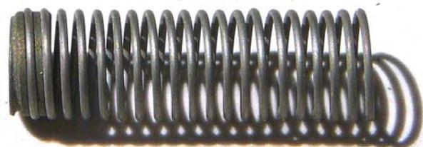
**Fig.4. The wolfram filament, thread-mounted on the molybdenum fixing piece, in order to be welded.**
