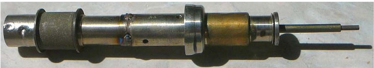
**Fig.1. Indirect-heated cathode, made by WIG welding (center) and by electron beam welding (left).**
