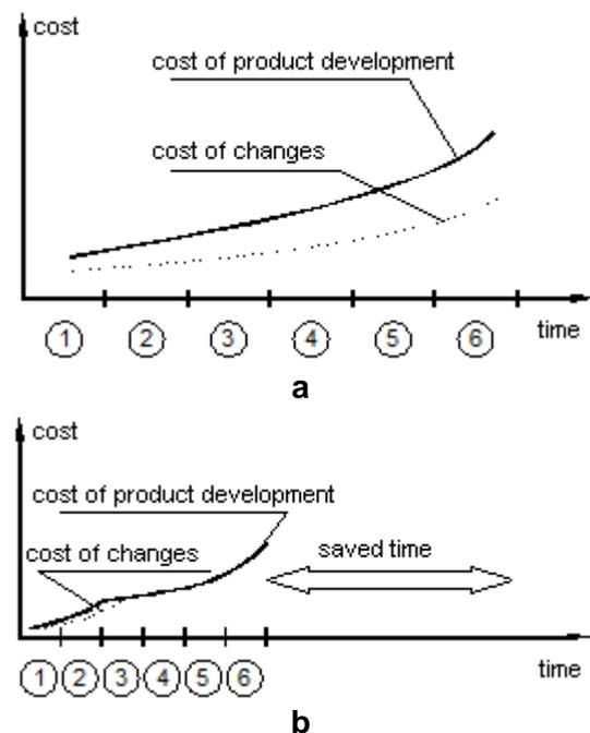
**Fig.1. Comparison between the classic development of a product (a) and use of RP technologies (b); 1 – idea, 2 – conception, 3 – finishing, 4 – elaboration of documentation, 5 – realization of verification tools and devices, 6 – production.**
