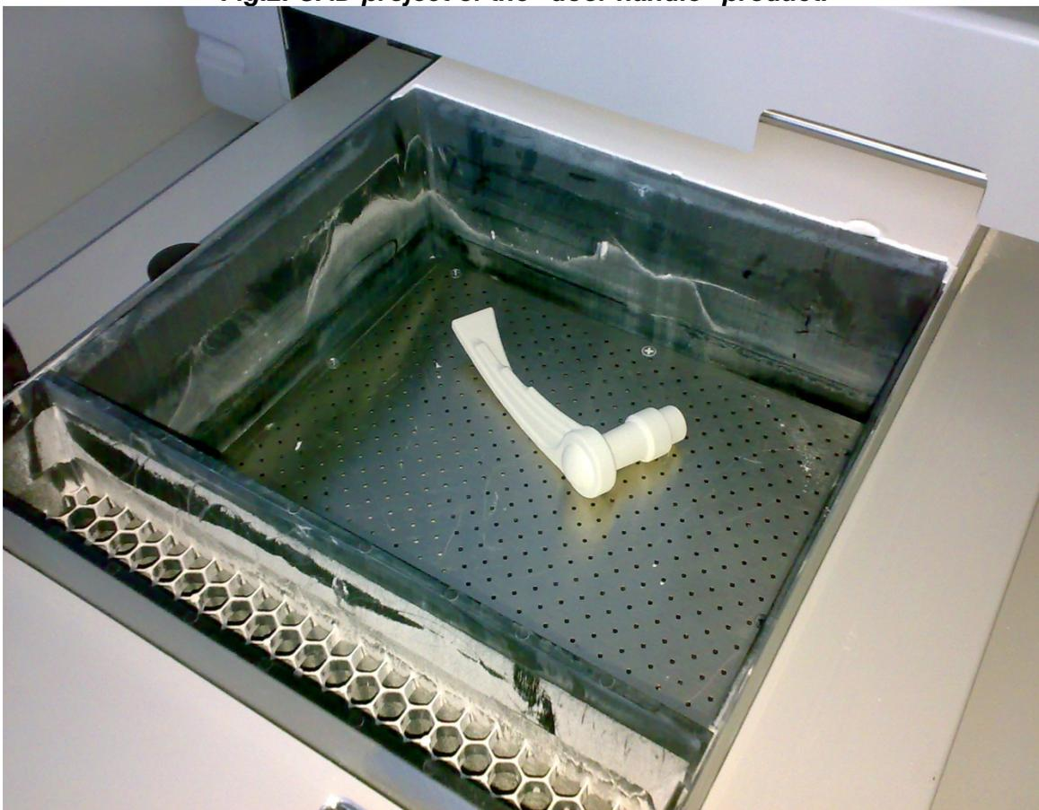
**Fig.3. Plastic prototype of product, made by 3D printing.**
