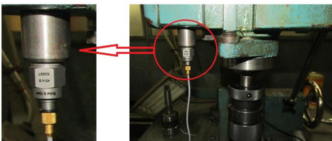
Figure 2. Mounting the vibration sensor
