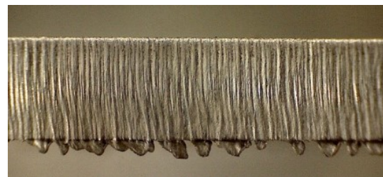
f) experimental trial 18 (P=3.5 kW, p=10 bar, v=3.5 m/min)
