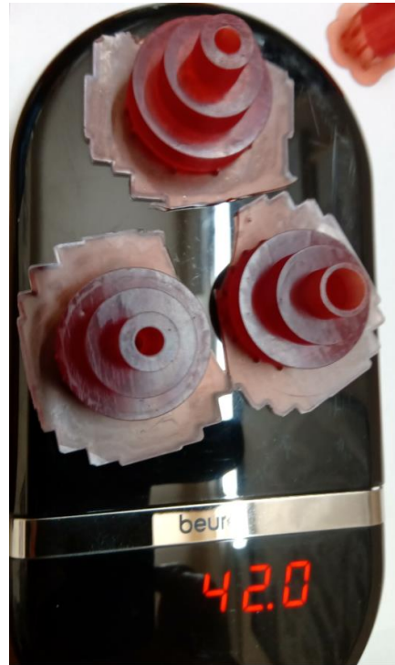
Figure 15. Multiple part for DLP printed with supports
