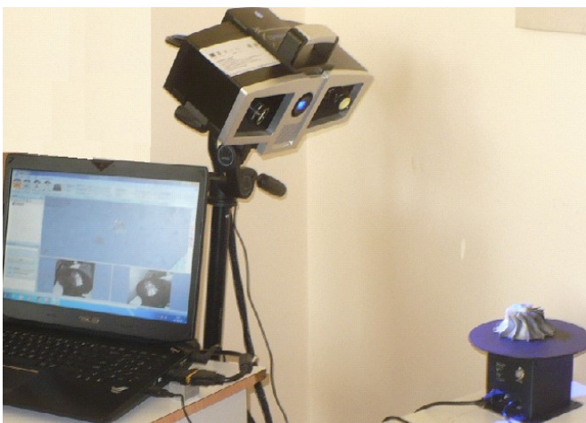
Figure 2. The 3D scanning system
