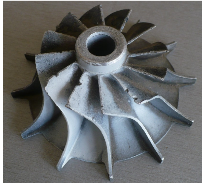
Figure 3. The worn impeller.
